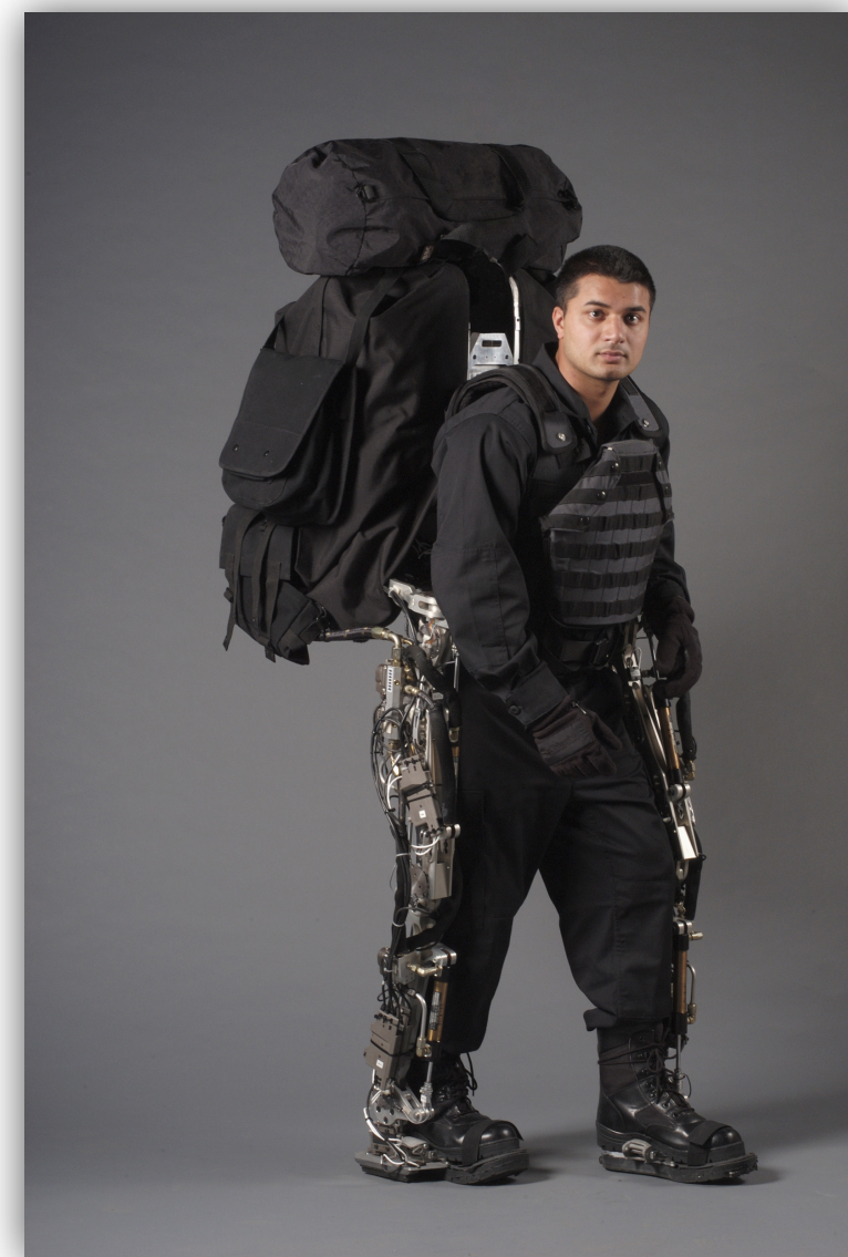
BLEEX-exoskeleton: for military and disaster relief personnel
